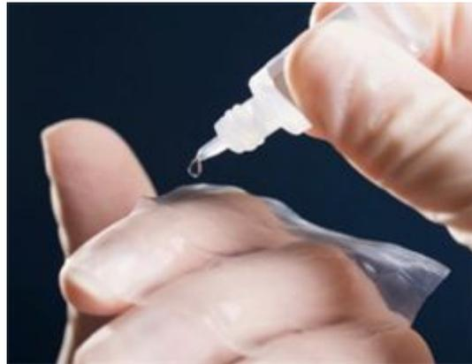
**2** Touchless, aqueous solution relaxes membrane onto delicate surfaces and geometries
