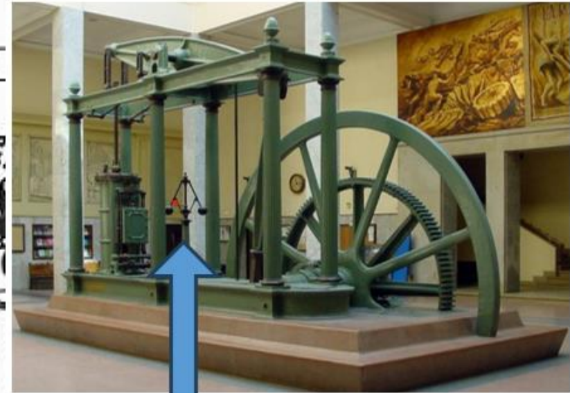
The fly-ball governor — a second innovation to keep the steam engine speed stable.
