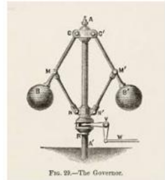
The fly-ball governor — a second innovation to keep the steam engine speed stable.
