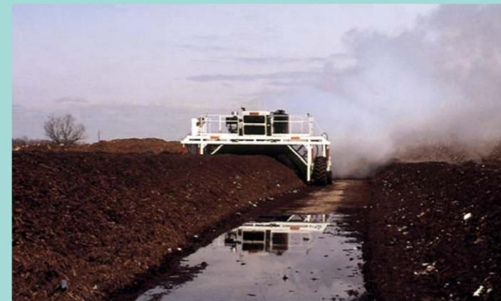
Biosolids are mixed with bulking materials and formed into windrows (long piles).
